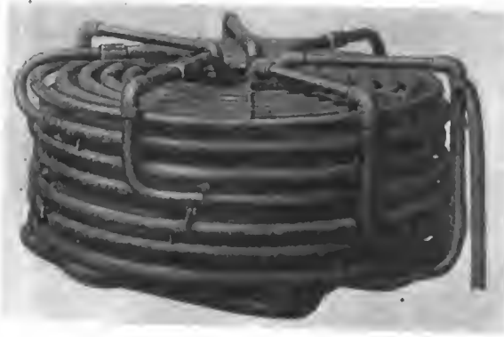
Steam Generator of the White Cars.
